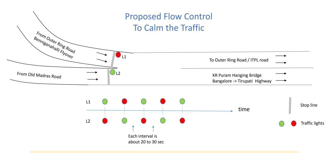
Achieve flow control using short-duration traffic lights which are synchronized.
